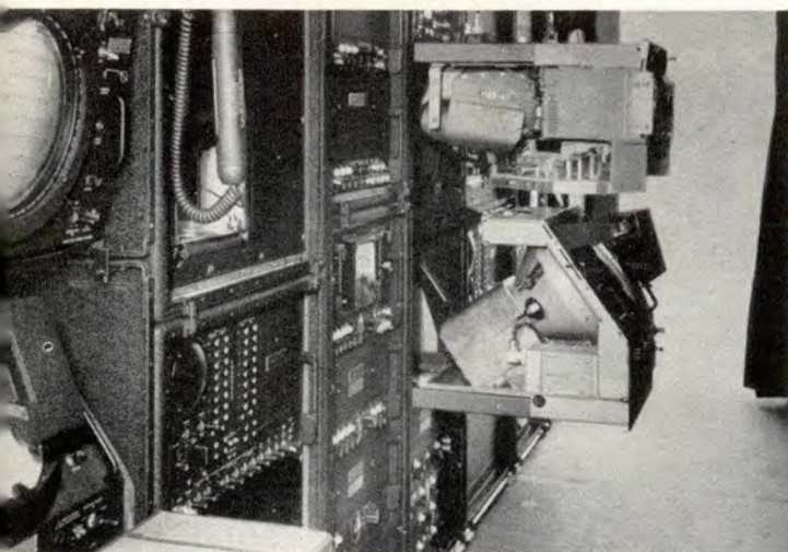
CPN-4 interior showing scopes pulled out from racks for maintenance. Accessibility is stressed throughout the new GCA units. Below, an operator checks air traffic on the GCA scope located in the control tower at the Los Angeles airport.
