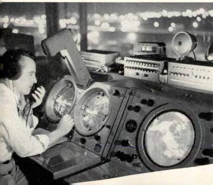
CPN-4 interior showing scopes pulled out from racks for maintenance. Accessibility is stressed throughout the new GCA units. Below, an operator checks air traffic on the GCA scope located in the control tower at the Los Angeles airport.
